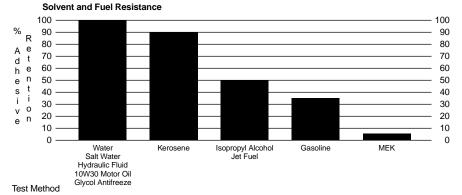
Tape between stainless steel and aluminum foil.
